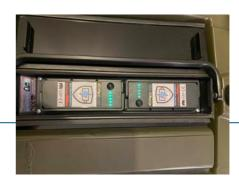
Push the battery tray lid down firmly, the circumferential sealing tape ensures that it is watertight.
