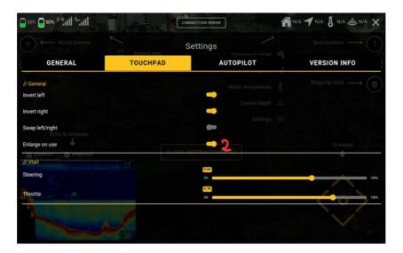
The settings marked 3 are settings with which you can set the sensitivity of the steering (top bar) and the maximum speed (bottom bar)
