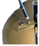
The "shark fin" ceramic antenna for the echo sounder is pushed down firmly at the rear.
